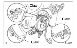
(c) Release the 3 claws and remove the spiral cable. **NOTICE:**
